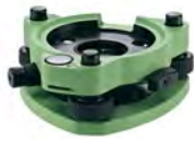
777509 Leica GDF322 Leica Professional 5000 green tribrach with optical plummet
