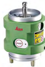
874838 Leica SNLL321 Precision carrier with laser plummet The laser provides convenient steering up even in conditions of poor visibility. Reflector centring accuracy 0.3 mm, plummet accuracy 1.0 mm at 1.5m.
