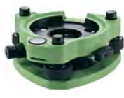
777509 Leica GDF322 Leica Professional 5000 green tribrach with optical plummet
