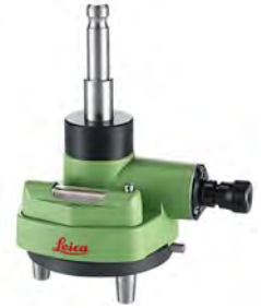
725566 Leica GZR103 Carrier with optical plummet. Rotatable carrier with longitudinal bubble for use in tribrachs without plummet. Reflector centring accuracy 1.0 mm, plummet accuracy 0.5 mm at 1.5 m.
