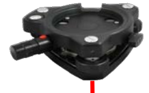
05-1300-B SitePro Eurostyle Tribrach with 8-min circular vial and laser plummet
