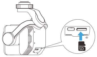
Fig 3-17 Installing the microSD Card
