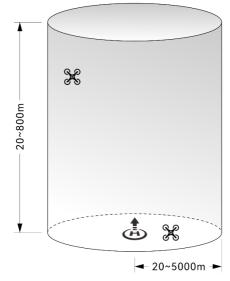
Fig 2-5 Diagram of altitude and distance limits
