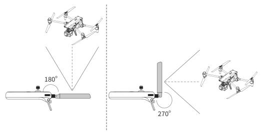
Fig 4-10 Extend the antenna
