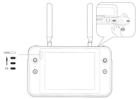
Fig 4-8 Checking the Battery Level of the Remote Controller
