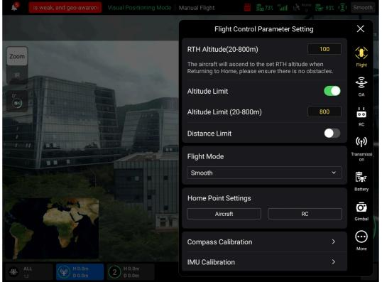
Fig 6-4 "Flight Control Parameter Setting" interface
