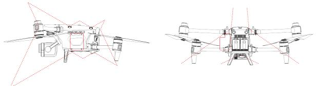
Fig 2-1 Mount gravity center and non-interference zone (circled by red line)
