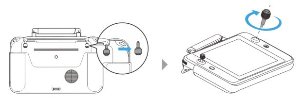
Fig 4-5 Installing command sticks
