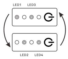
Fig 5-5 Self-heating State
