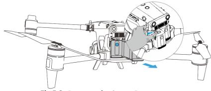
Fig 5-3 Remove the Smart Battery
