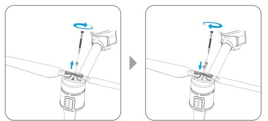
Fig 3-7 Install the Propellers
