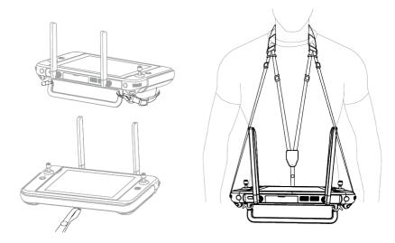
Fig 4-4 Install the Remote Controller Lanyard (As Required)
