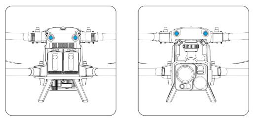
Fig 2-2 Front and rear visual lens modules of the aircraft
