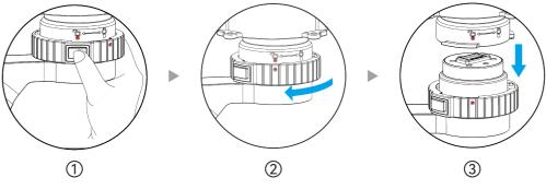
Fig 3-16 Removing the Gimbal
