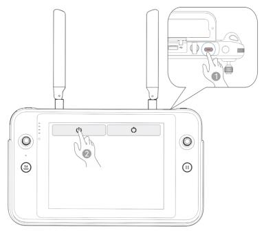
Fig 4-7 Turning the Remote Controller Off
