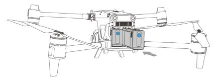
Fig 5-2 Install the Smart Battery
