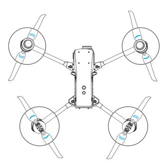
Fig 3-6 Aircraft Propeller Mounting Layout (silk printings are oriented toward the top of the fuselage)
