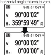
Selecting the direction of horizontal angle measurement.
