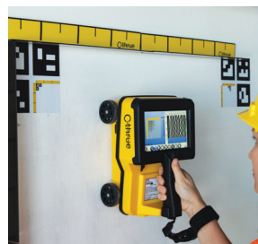
Automatic position and navigation system (Virtual Pad) increases productivity and reduces survey times.
