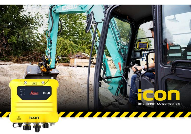
The Leica CR50 communication unit supports an internal cellular modem and a dual-frequency radio. The Leica CR50 can be connected to the iCON gps 100 on-machine GNSS receiver to perform high-accuracy RTK GNSS positioning.
