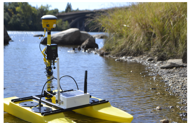
Unit can be integrated into remote / autonomous survey vessels
