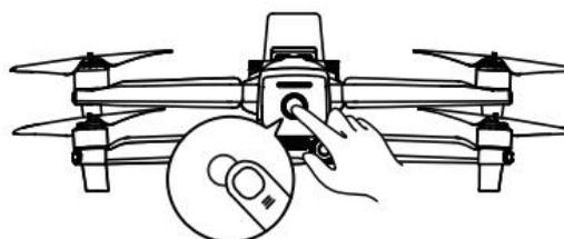
3. Press the remote controller pairing button for 3s at the right lower part of the aircraft. The pairing indicator flashes rapidly, indicating that the aircraft is prepared to be paired with the remote controller.
