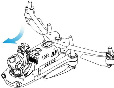
1) Please make sure that the ring at the front end of the gimbal is aligned with the two pins in the gimbal compartment of the machine head.
