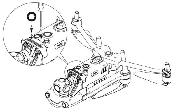
4. Turn on the power switch of the aircraft. If the connector cable of the gimbal is connected correctly, the gimbal will rotate automatically to carry out self inspection.
