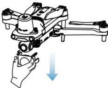
After the aircraft is used, the gimbal protective cover shall be reinstalled to prevent the gimbal from damage.
