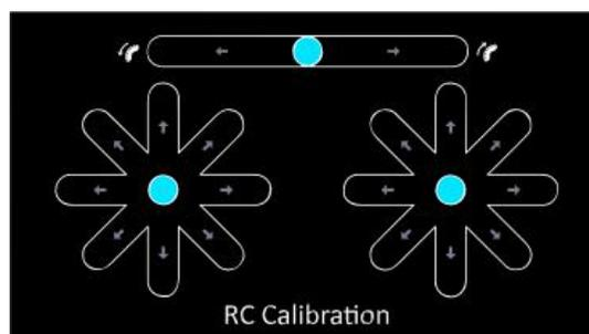
3. Push and hold the **rocker** in eight directions one by one until you hear a beep. Then turn the **gimbal pitch angle knob** clockwise until you hear a beep, and turn it counterclockwise until you hear a beep.
