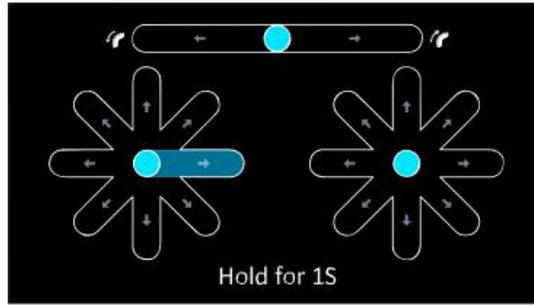
4. Push and hold the **rocker** in eight directions one by one until you hear a beep. Then turn the **gimbal pitch angle knob** clockwise until you hear a beep, and turn it counterclockwise until you hear a beep.
