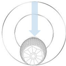
Push the left rocker to the bottom and hold in the position for 2s
