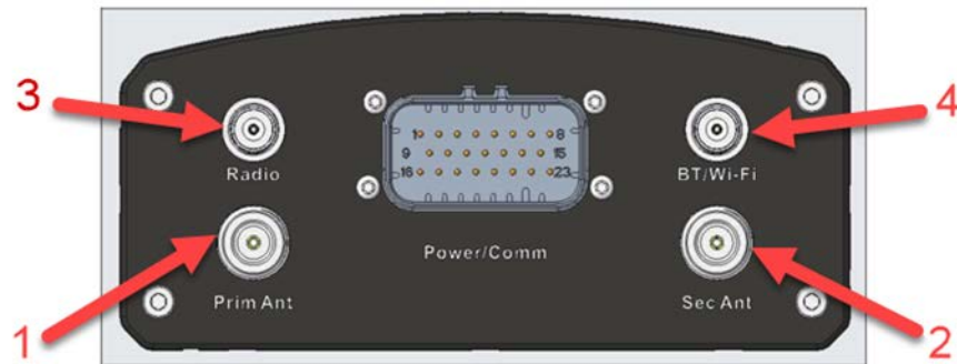
Figure 2-7: VR1000 back panel and pin-out
