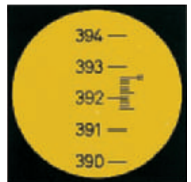
NAK2 circle reading (400 gon) 392.66 gon
