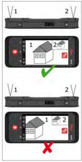
The photos from the two cameras are displayed on the BLK3D screen. Only points which are visible in both photos can be measured.
