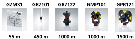
Figure 7 - Achievable ranges 1 for automated target aiming (static).
