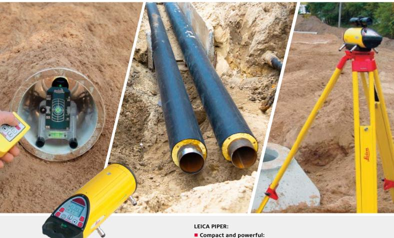
Solid performance in the pipe, over the top or in the manhole. The Leica Piper series helps you to work with confidence having the perfect instrument for your application and need. Built with a rugged aluminium housing, these pipe lasers perform powerfully even in tough jobsite conditions.
